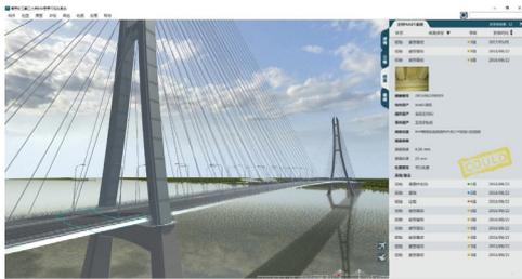
With component IDs as the index, the geometric models and data were all linked in the Unity database (based on the division and basic information of the IFC standard), with all of the component's original geometric dimensions, positions, relationships, and attributes restored.
